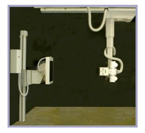
Wall stand with vertical sliding and tilting frame for digital receptor 41x43 cm. Manual tilting at any position and autopositioning by motor at  $0^{\circ}$ .  $90^{\circ} + 20^{\circ}$ . Manual rotation with locking at  $0^{\circ}$  and 90 of the support frame, allowing proper grid orientation. Easy port access to interchangeable grids for compatibility with different focal distances. One plastic grid Frame included.
